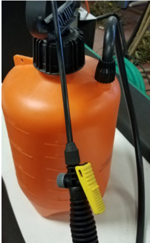
A pump sprayer is ideal for delivering low pressure to specific points that need cleaning. A high pressure washer would splash debris deeper into the equipment, splatter debris onto food contact surfaces all over the facility, and can atomize contaminants that can cross contaminate elsewhere.
