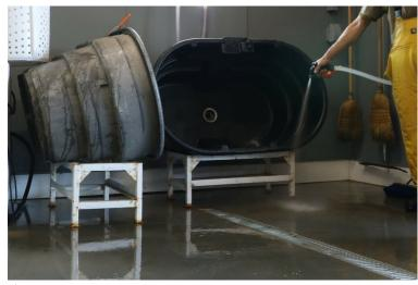
This farm uses metal stands for their wash tanks. The stands keep the tanks off the floor during washing and drying and can even be moved with a pallet-jack even when full of water.
