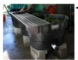
Stock tanks, on cinder blocks for prototyping to find the best working height. Note the use of coated, wire closet shelving above the tanks for holding and draining baskets.
